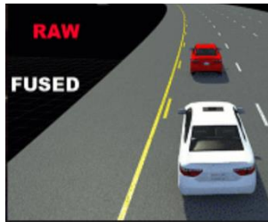
Ego vehicle localization using GPS and IMU fusion for Scenario Generation
