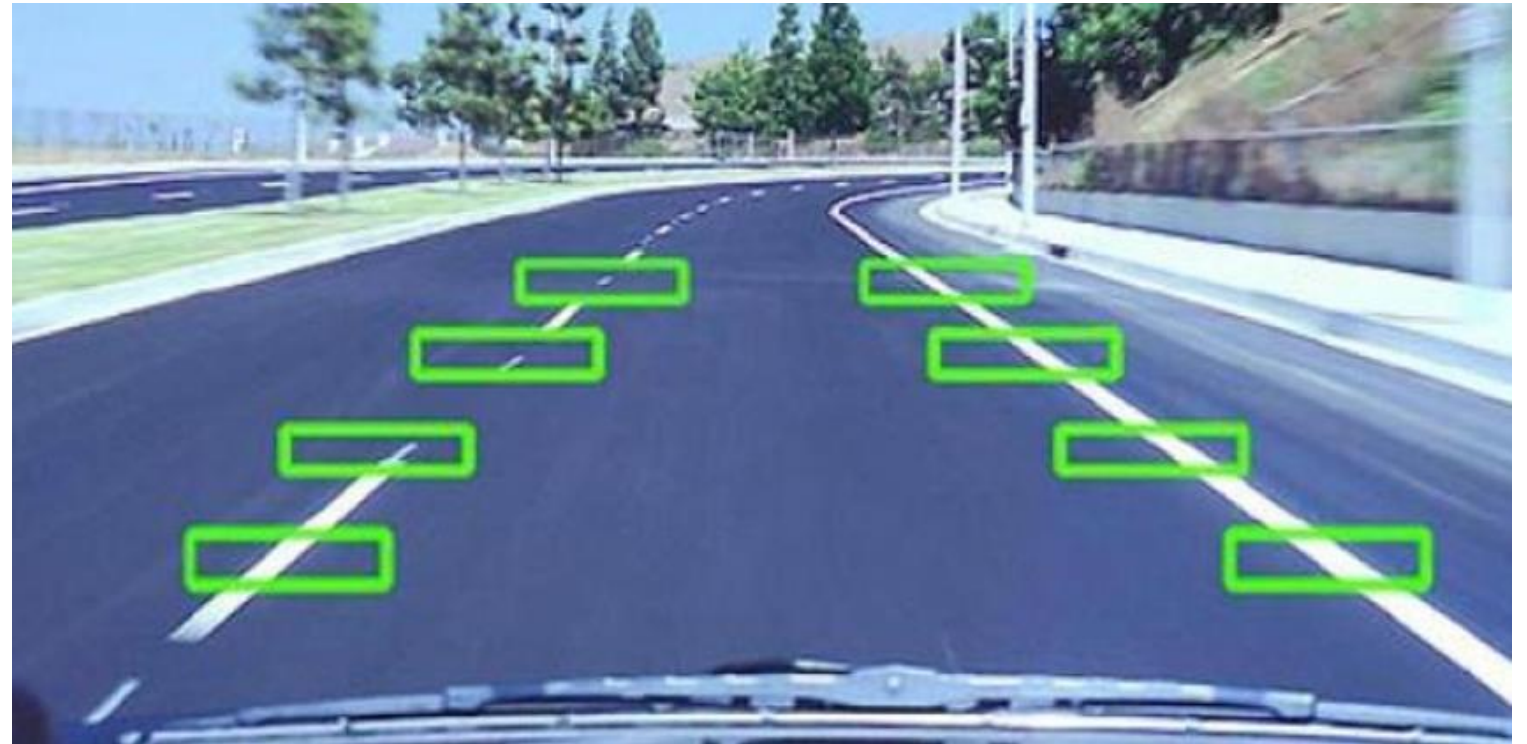
Mercedes-Benz Actros Lane Departure Warning System
