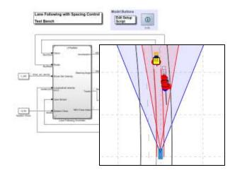
Lane Following Control with Sensor Fusion and Lane Detection
