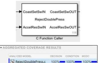
Custom C Code Verification with Simulink Test
