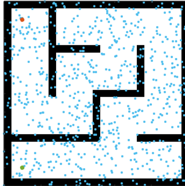
Uniformly Sampled space (used by conventional motion planning algorithms e.g., RRT/ RRT*)
