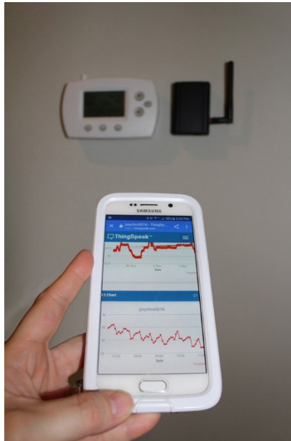
Figure 9. Internet of Things system using ThingSpeak for collecting and analyzing energy data.
