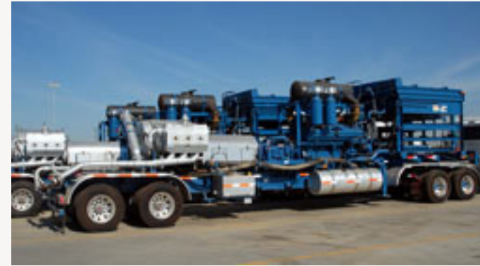
Truck with positive displacement pump.
