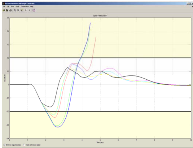
Figure 6: Evolution of the estimated slip angle signal as the automated tuning process evolves.
