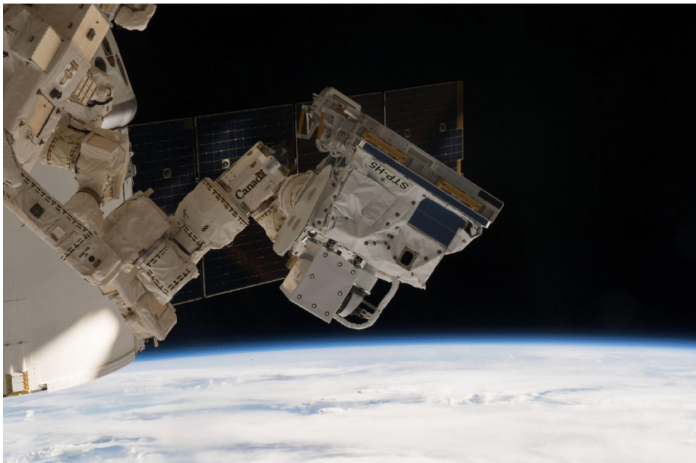
NASA's Raven deployed on the International Space Station. Raven is an on-orbit testbed for developing vision-based sensing systems for relative navigation. Image courtesy NASA.
